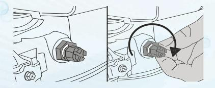
Then measure the water hardness present on the outlet of the system and check that it fits within the desired values. Otherwise adjust regulator and check again
