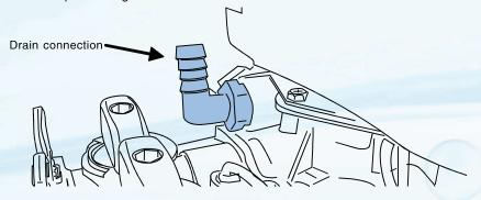
The overflow hose of the system must be driven towards a nearby drain outlet. Under no circumstances should this pipe be on a higher level.
