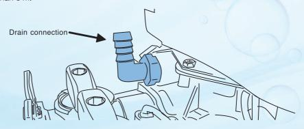
The overflow hose of the system must be driven towards a nearby drain outlet. Under no circumstances should this pipe be on a higher level.
