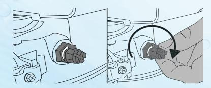
Then measure the water hardness present on the outlet of the system and check that it fits within the desired values. Otherwise adjust regulator and check again
